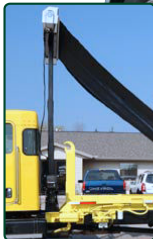
• Housing Surrounds Tarp & Spool For Protection Tower Adjusts 60" From Rest Position Up to 117"
